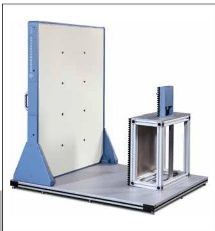
concept that is geared specifically to testing automotive radomes.
