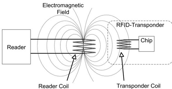
Figure 2: Working Principle
