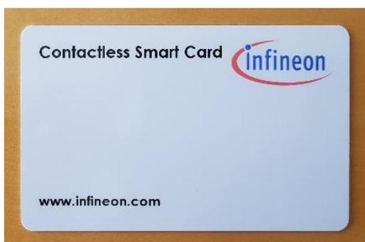
Figure 1: ID-1 Infineon smart card (Class 1)
