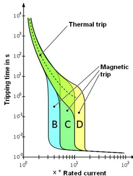
Fast tripping is important, because when the 24 V DC supply fails the intact branches are also undersupplied. Voltage interruptions of 20ms are already critical for the PLC and will cause the process to be interrupted or even to crash.
