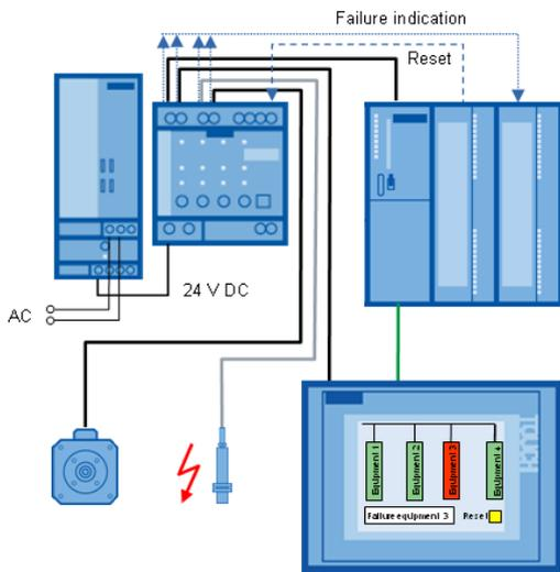
Application example with a standard power supply (for example, from the SITOP smart product line) and selectivity module SITOP PSE200U:
