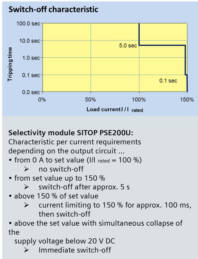
**Extensive functionality assures a targeted fault localization**
