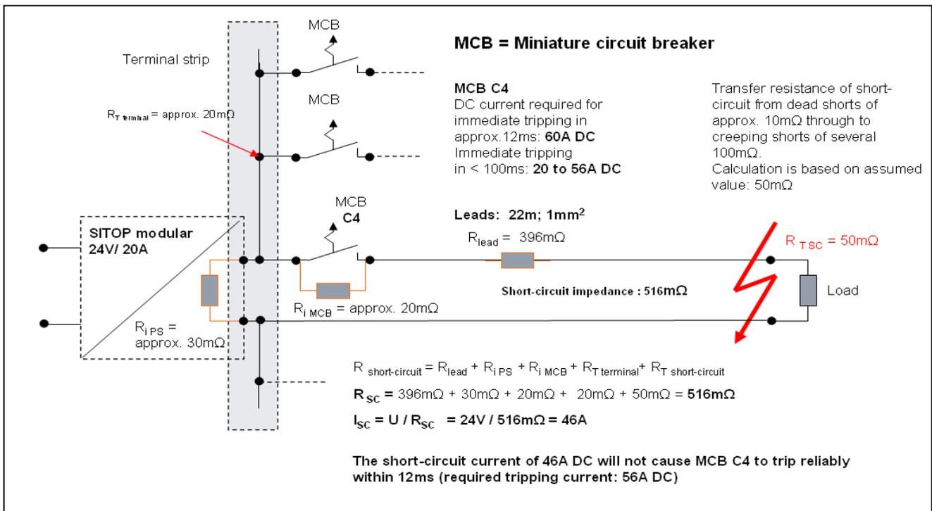
**Application example with limited short circuit current**
