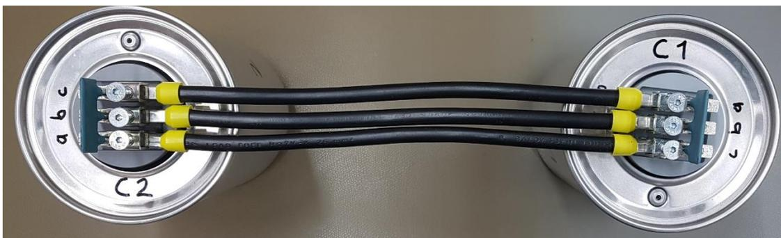
Figure 11: MTFC parallel connection
