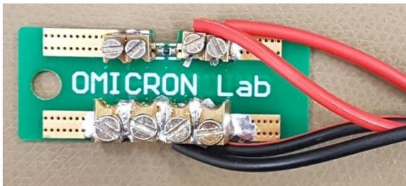
Figure 6: Open calibration
