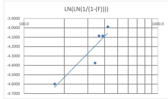
Data was fitted to the Weibull distribution using JMP Software (version 13) using Maximum Likelihood. The shape parameter  $m = 0.74$ . This value for the shape parameter will then be used to calculate the PPM quality level, as follows in this document.
