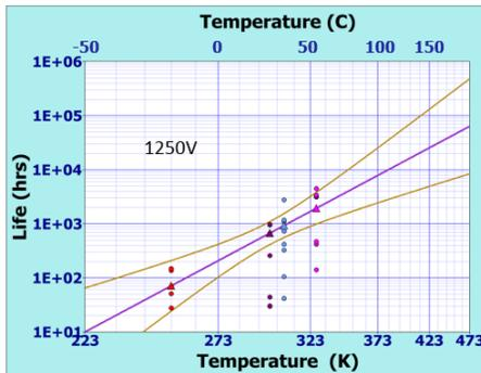
The slope of the plot as analyzed with Alta-pro software reveals the activation energy  $E_a = -0.3eV$  and the acceleration
