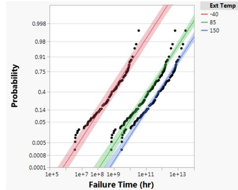
This use plot of the data which shows that even at  $-40^\circ$  C @480V wear out of the device does not begin before  $10^6$  hours.
