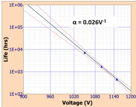
A linear TDDDB (time dependent dielectric breakdown) model was used, which is a conservative model relative to ttf (time to fail). In other words this model results in the shortest lifetime. The Voltage Acceleration Factor ( $AF_V$ ) is defined in (1), where  $\Delta V$  is the difference between the stress voltage and the usage voltage.
