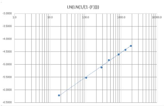
Based on this calculation is reasonable to assume that we are in the “bottom” of the bathtub curve, and can use this assumption in calculating FIT rates.
