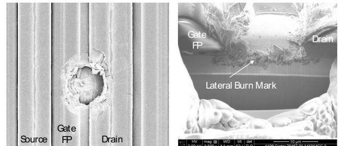
This failure mode dominates the off state failures regardless if the failure is caused by voltage or temperature acceleration. It shows up as wear out failure (intrinsic) and also shows up as
