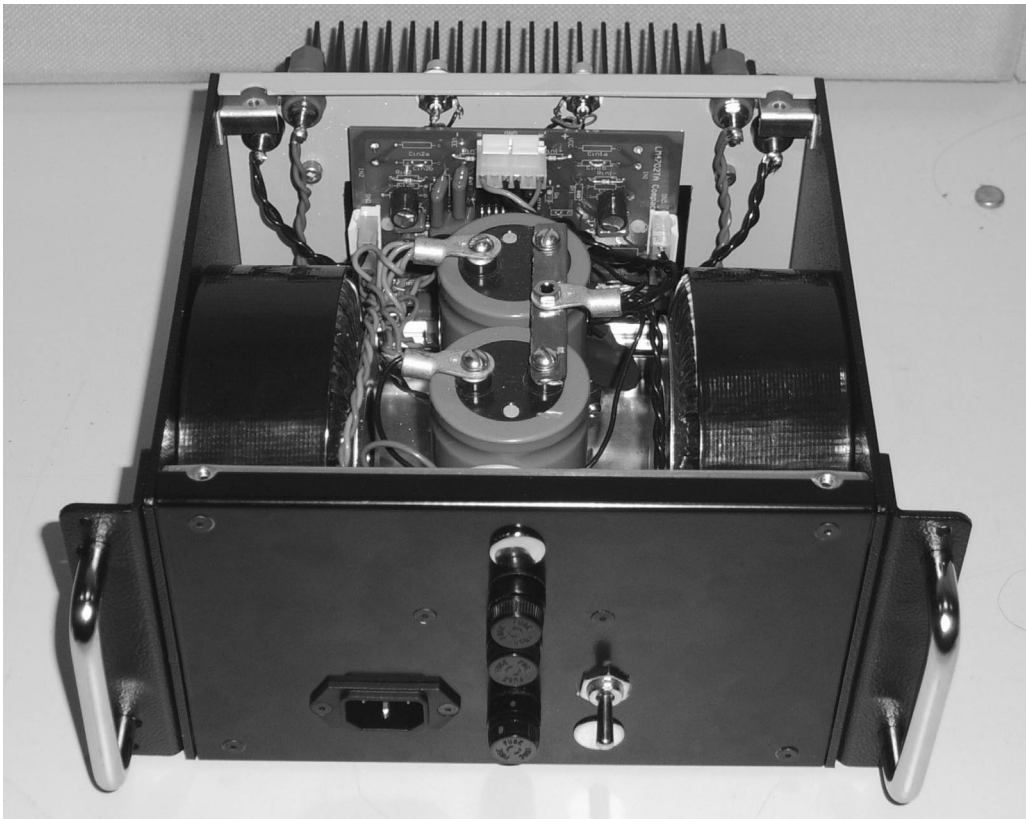
FIGURE 1. Complete LM4702 – based 100W/channel High-Fidelity Power Amplifier
