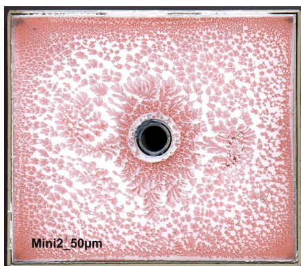
Fig. 11: Bottom view with satisfactory thickness of paste layer
