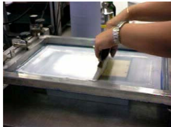
Fig. 7: Filling the mesh with paste
