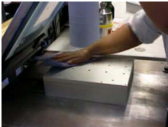
Fig. 6: Cleaning the heat sink
